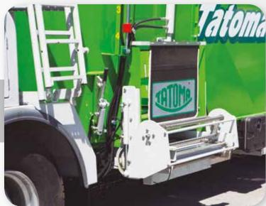
The cutter rotation direction is reversible thanks to the two electric drive pedals that allow more precise control of the load, as loading can be stopped and the excess product returned on reaching the required amount.
