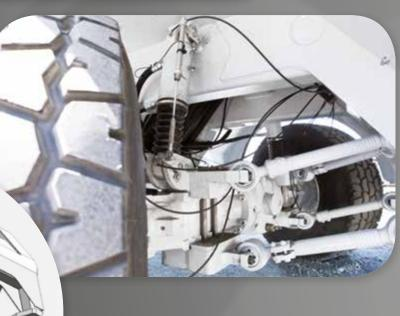
Front-axle levelling is performed by a hydraulic suspension. The two rear-axles are connected by a tandem chassis with leaf spring and rocker suspension. The first axle is for steering and driving, the second for driving and the third for steering, allowing the machine exceptional manoeuvrability despite its size. The maximum turning angle is 40 °. The service brake is located on the first and second axle and measurements of all wheels are 445/65 R22.5
