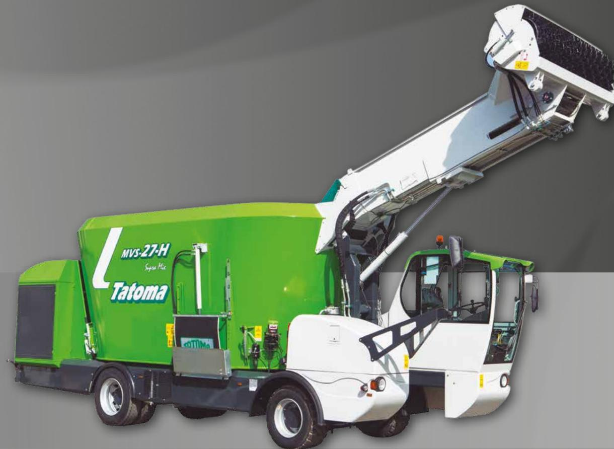
Front-axle levelling is performed by a hydraulic suspension. The rear-axle is connected by a chassis with leaf spring and rocker suspension. The first axle is for steering and driving, the second for driving and steering, allowing the machine exceptional manoeuvrability despite its size. The maximum turning angle is 40°.
